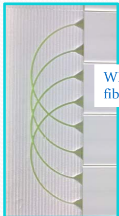
Extruded scintillator bars 160cm long
